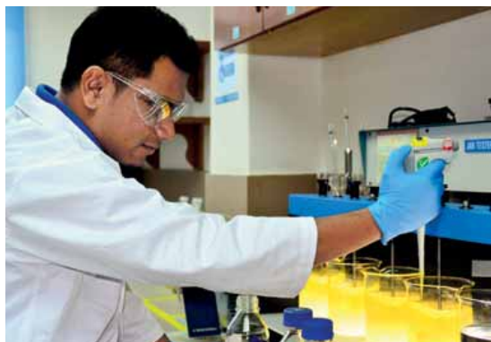
Jar testing to determine optimum coagulant dosage at Central Laboratory
